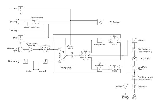
Figure 2.6 T826/827 Audio Processor Block Diagram
