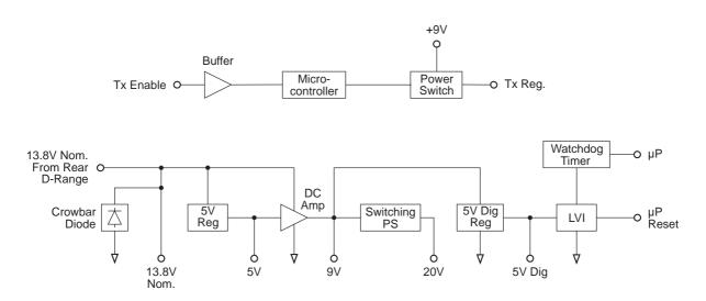
Figure 2.7 T826/827 Power Supply & Regulators Block Diagram
