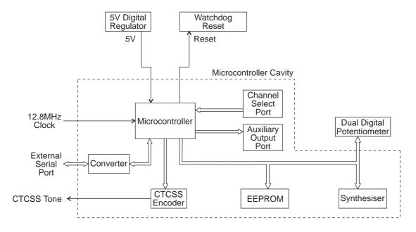
Figure 2.3 T826/827 Microcontroller Block Diagram
