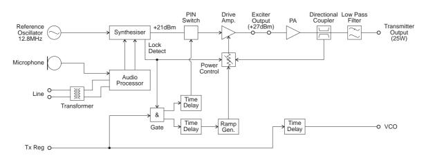
Figure 2.1 T826 High Level Block Diagram
