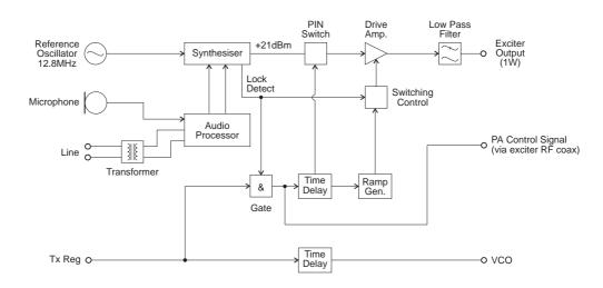
Figure 2.2 T827 High Level Block Diagram
