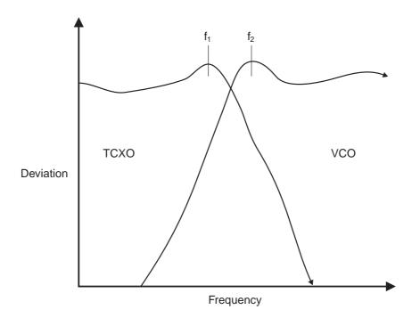
Figure 2.5 T826/827 Two Point Modulation
